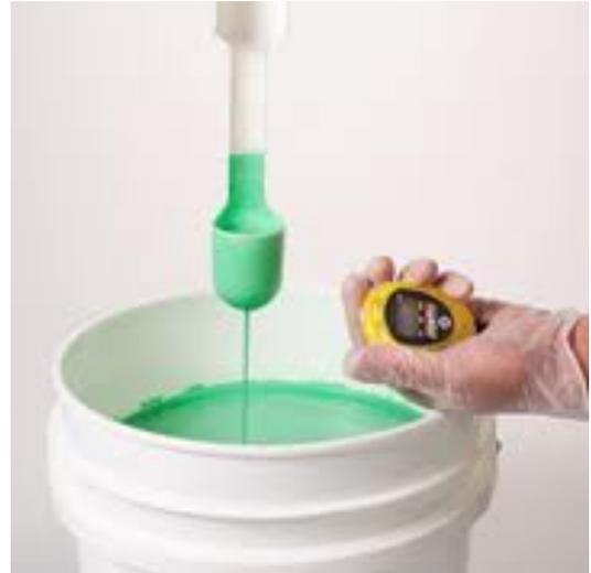
A viscosity cup is a simple tool for measuring the viscosity of flowable paints and liquids
