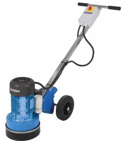
A larger diameter buffing machine can be used to take the concrete from a honed to a polished finish
