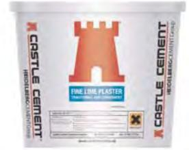
Castle Fine Lime Plaster is a traditional 1: 2 lime: sand wet mortar mix. It is produced using silver sand, soft sand and non-hydraulic (fat or pure) lime derived from high calcium quicklime (CaO) slaked and stored for a minimum of 30 days.
